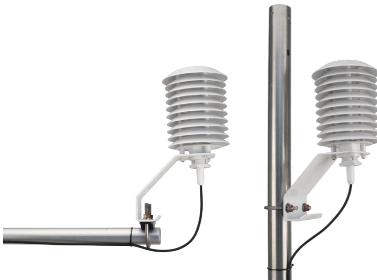
Figure 7-1. HC2AS3 and 41003-5 Radiation Shield on a CM200 Series Crossarm (left) and on a tripod mast (right)
