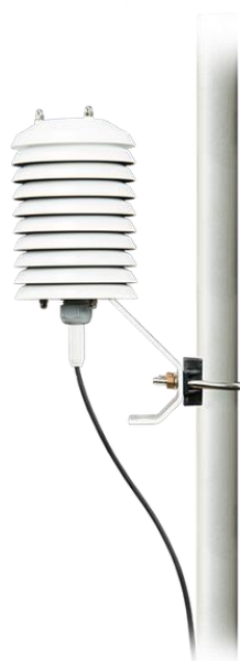
Figure 7-2. HC2AS3 and RAD10 Radiation Shield on a tripod mast
